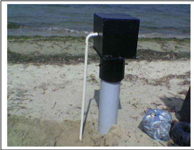
Shallow borewell with float sensor. The cable connecting the float sensor to the 15-channel Water Level Recorder passes through the plastic pipe.
