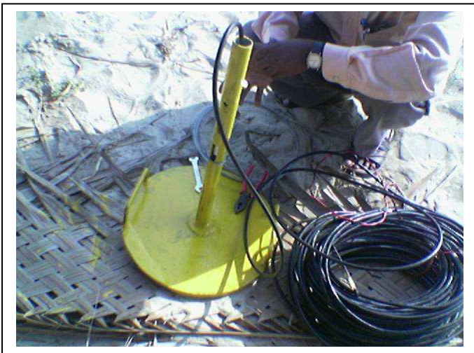
Pressure transducer introduced into the hollow pipe connected to the dead weight to be installed on the shallow sea floor 15 m inside the water front.
